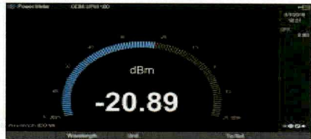
Optical power measurement trace (R&S®FPH-K9)
